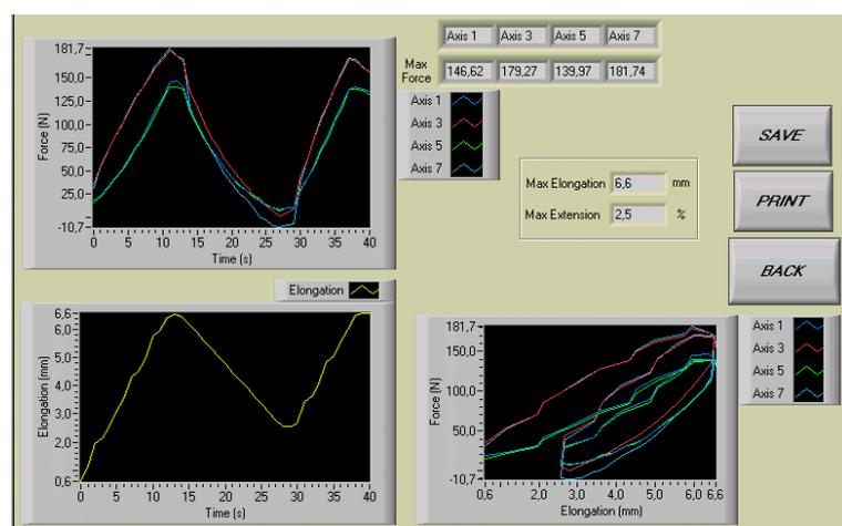
Fig. 5 - Fatigue test: The number of cycles as well as the elongation and force are independently programmable
