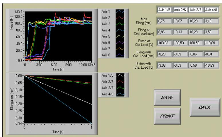
Fig. 6 - CRL Test under multiaxial loading (for the 8 actuators over the 4 axes)
