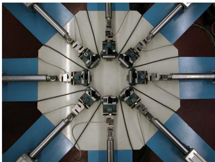
Fig. 1 - Top view of TexTest equipment
