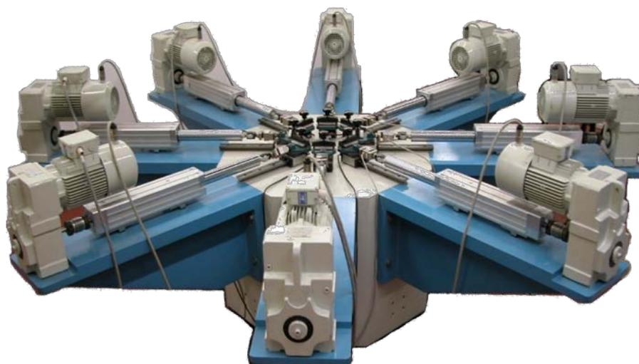
Fig. 2 - TexTest multiaxial testing equipment
