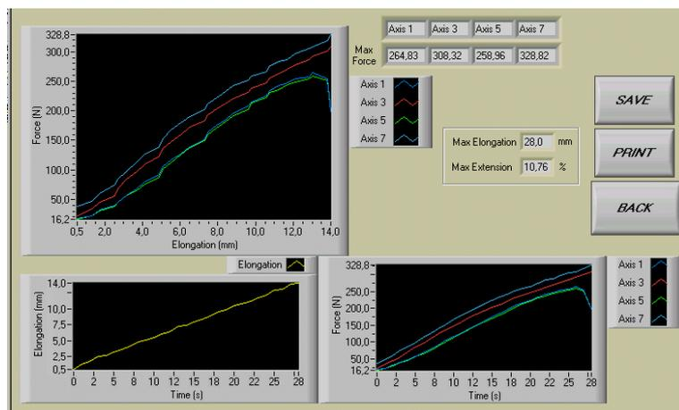
Fig. 4- CRE Breaking test under biaxial loading
