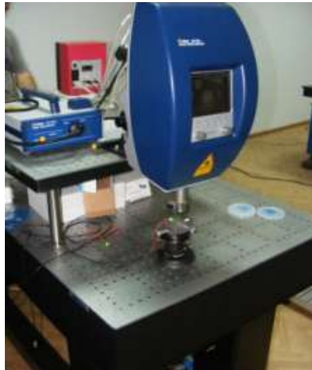
Figure 1: Differential laser vibrometer and optical head of the MSA-500 system
