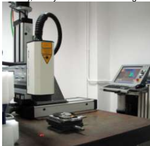
Figure 4: The structure of the dynamic analysis system of the miniature structures through 3D laser vibrometry: robotized positioning system and laser vibrometer with 3 concurrent laser beams 3D based on Doppler Effect
