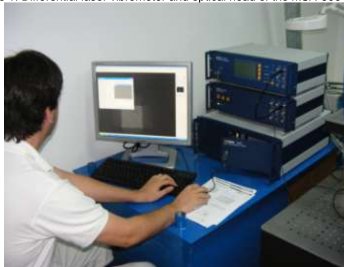
Figure 2: Command, data acquisition and post-processing unit, junction box and decoder of MSA-500
