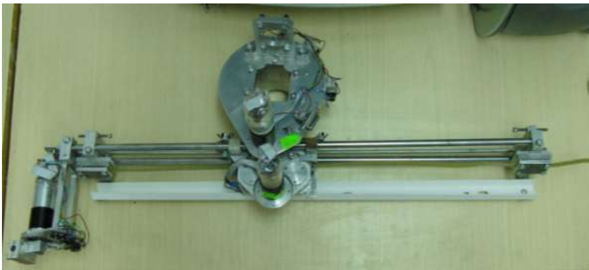
Figure 6: Robot for vibro-acoustic scanning – orientation system
