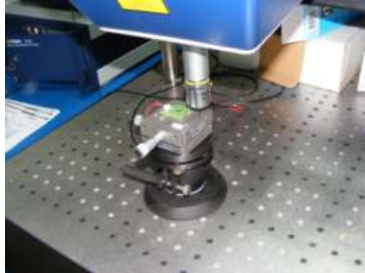
Figure 3: Dynamic testing of a MEMS type positioning system with electrostatic actuator using the MSA-500 system
