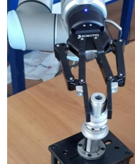
Figure 4. UR10 manipulator robot with 2F-140 adaptive gripper
