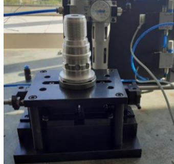
Figure 3. Inner diameter measurement system
