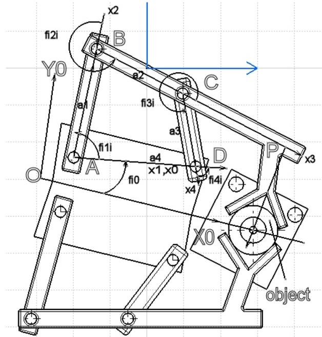
Fig. 1. The model of the compliant gripper.
